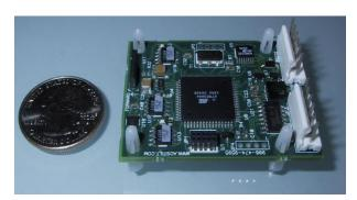
Low cost SOLID STATE advanced Pitch / Roll / Temperature compensated COMPASS / MAGNETOMETER system is built around a state of the art CMOS microcontroller utilizing AOSI's proprietary algorithm on a 1.5" x 2" assembled PCB with a total height including tilt sensing elements of less than 0.5".
